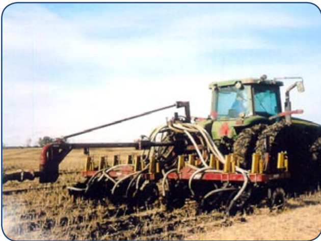
Manure injector showing distribution manifold and trailing deliver hose.
