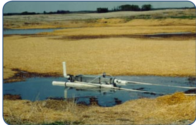
Odour collection from an earthen manure storage.
