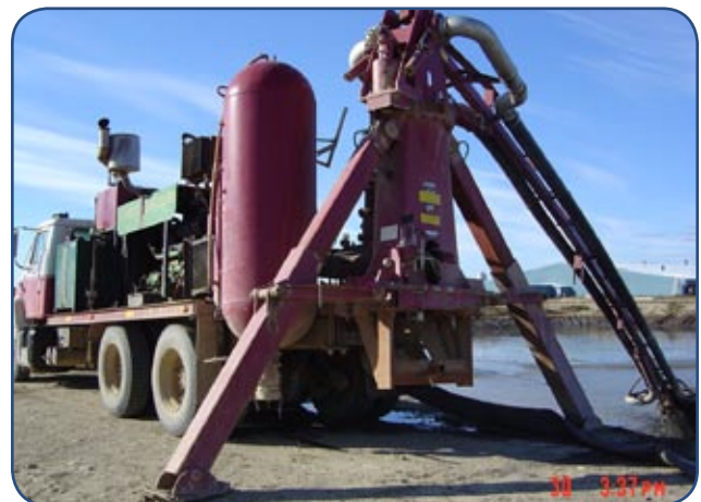
Main manure delivery pump to the field injection unit.
