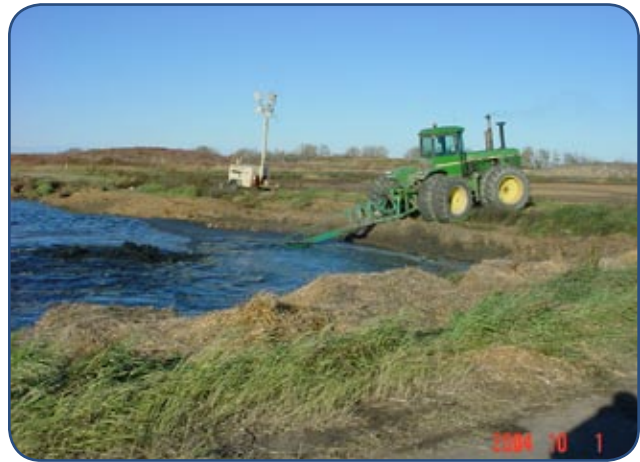
Agitator at earthen manure storage.
