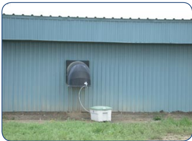
Continuous air sampling from an exhaust fan using a peristaltic pump.
