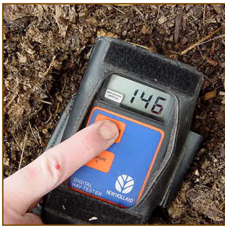
Figure 6: This pile is at an optimum temperature of 146 F (63 C)
