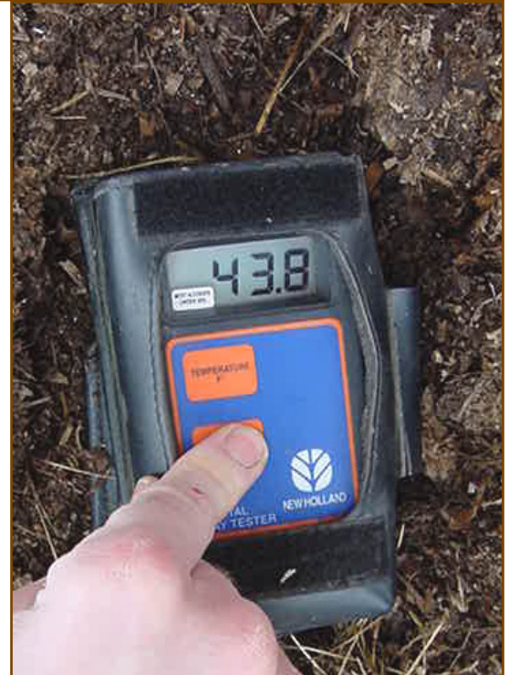
Figure 5: A hay moisture probe with a long stem works well to measure the moisture content of a compost pile. This pile is at the correct moisture level of about 45 per cent.
