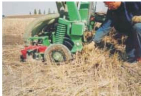
Low disturbance injection typically refers to the use of coulters to open the soil.
