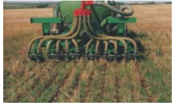
Coulter-type injection equipment allows low disturbance liquid manure injection into forages.
