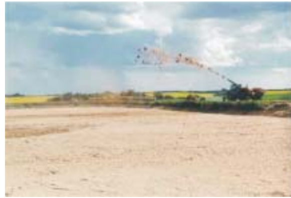
The Top Gun blowing straw onto a manure lagoon. Photo Courtesy: PAMI
