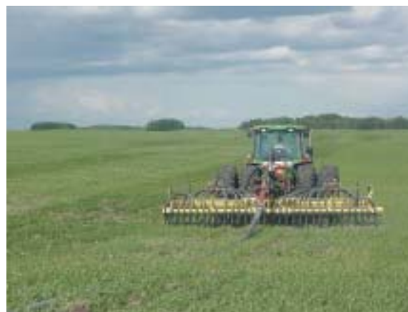
In-crop manure application to spring wheat using an Aerway applicator and drag line system.
